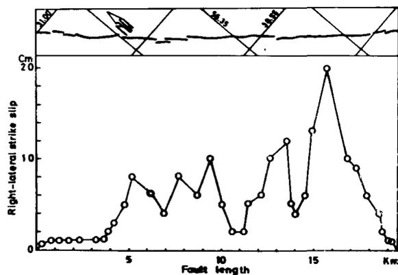
Fig. 5. Inconsistent horizontal displacement at the surface along the Bob-Tangol earthquake fault of 19 December 1977. Vertical axis is right-lateral displacement in centimetres and horizontal axis is fault length in kilometres.
